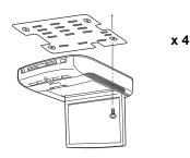
\*1 Installation Bracket is used to stabilize the monitor at the time of installing the monitor. Ask ALPINE dealer for detail.
